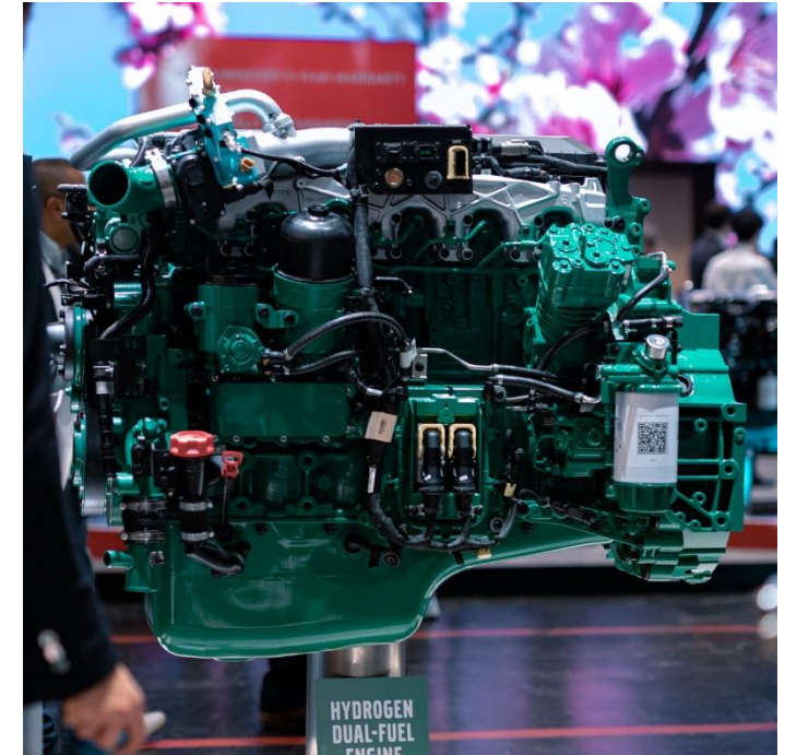
Dual fuel (hydrogen/diesel) solution for combustion engine in partnership with CMB.Tech
